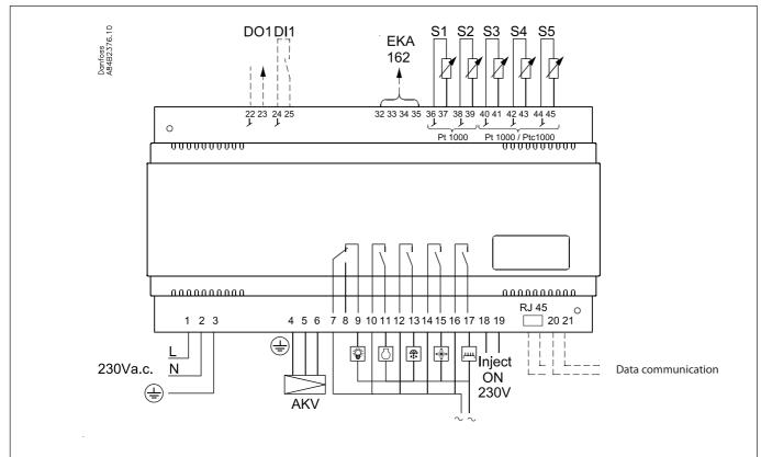
Cable length between an external display (EKA 162 or EKA 161) and EKC 514B1 must be max. 15 m
